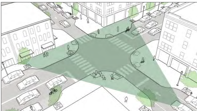
Example diagram of intersection visibility. Source: NACTO
