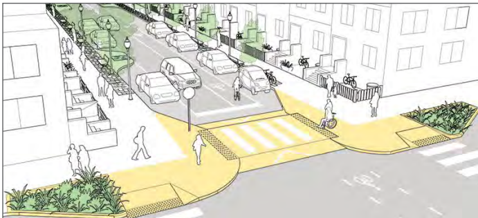
Example of a raised crossing. Source: NACTO
