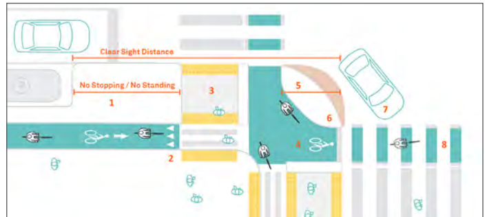
Diagram of a corner of a protected intersection. Source: NACTO
