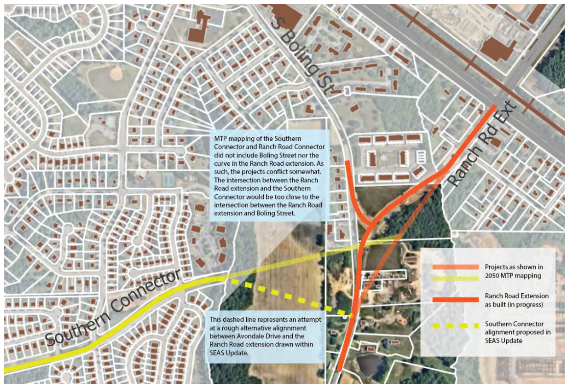
Diagram showing conflict between the Ranch Road Extension and the 2050 MTP version of the Clayton Southern Connector. Draft SEAS Update recommendations include a suggested modified alignment to address this, but further design/engineering is needed to refine alignment
